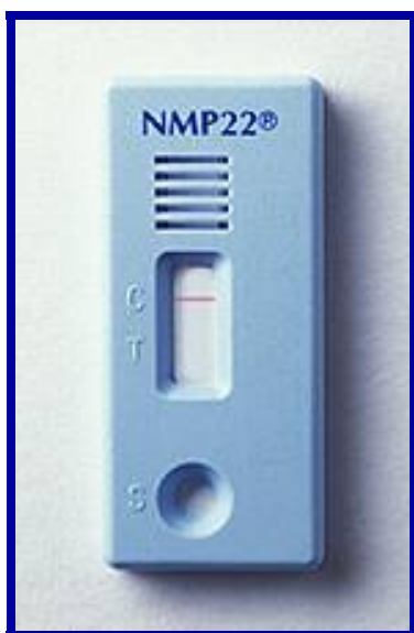
Figure (Left) - BladderChek Test, shown actual size. Dimensions are approximately 2 1/2 x 1 1/8 x 1/16 inches (67 x 29 x 6 mm). The urine specimen is introduced in the circular specimen port ("S", bottom arrow). The results are read 30 minutes later in the rectangular window (top arrow). In this example, there is a line visible at the mark "C" (for control), but no line at the position marked "T" (for test). This indicates that the test worked properly (control line present), but that NMP22 was not detected (no line at T). This would be a negative result, that is, bladder cancer is not present.
